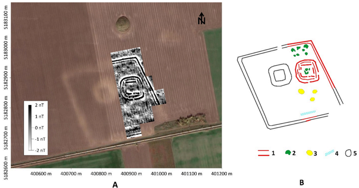
Fig. 7. Fort Kamianka V. (A) – magnetogram in greyscale and dynamics of the total magnetic field \pm 2.0 nT, black is high, placed on a satellite image; (B) - interpretation scheme: 1 – moats, 2 – dugouts, 3 – limestone structures, 4 – modern road, 5 – objects interpreted from the satellite image (after K. M. Bondar).
