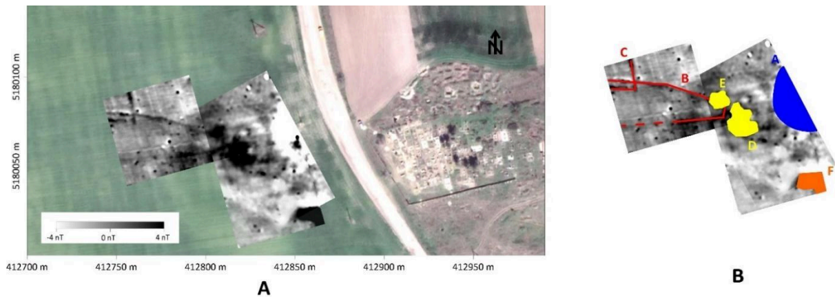
Fig. 6. Katalyne ashmound. (A) – magnetogram in greyscale and dynamics of the total magnetic field \pm 4.0 nT, black is high, placed on a satellite image; (B) – interpretation scheme explained in the text (after K. M. Bondar).
