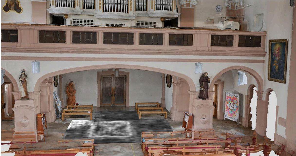
Fig 8. Overlay of 3D-model of the entrance area in the south of St. Margareta with the GPR depth slice of 7 ns depth showing the ribbed vault of crypt. View from North. White = high reflection amplitude, black = low reflection amplitude.
