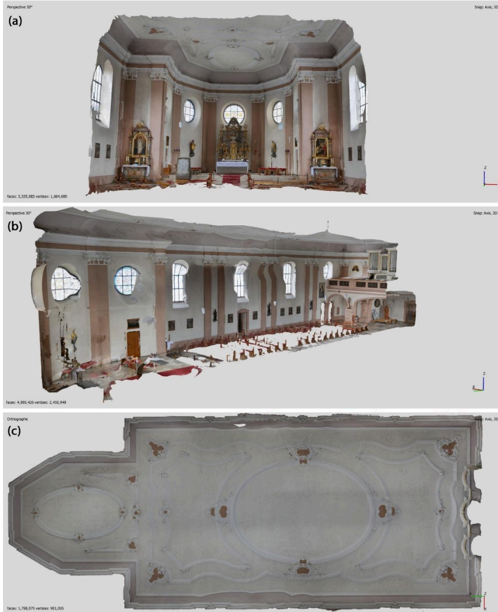
Fig 7. Three example views of the three-dimensional SfM model of the interior of St. Margareta in Kahl am Main showing the layout of the walls and the decoration as well as the mentioned problems. (a) Chancel, (b) Eastern half of the nave, view from Northwest, (c) Ceiling.
