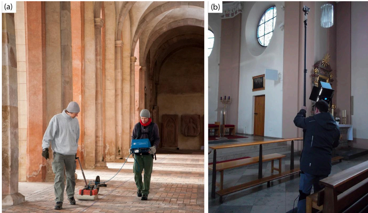
Fig 3. (a) Photo of the GPR-instrument GSSI SIR-3000 with 400 MHz antenna and odometer mounted onto a sled during a survey at the Monastery Eberbach im Rheingau (Photo: Jan Bosch, PZP), (b) Panasonic GX-800 camera mounted to the high-pole during the SfM survey inside St. Margareta Kahl am Main (Photo: Tatjana Gericke, BLfD).
